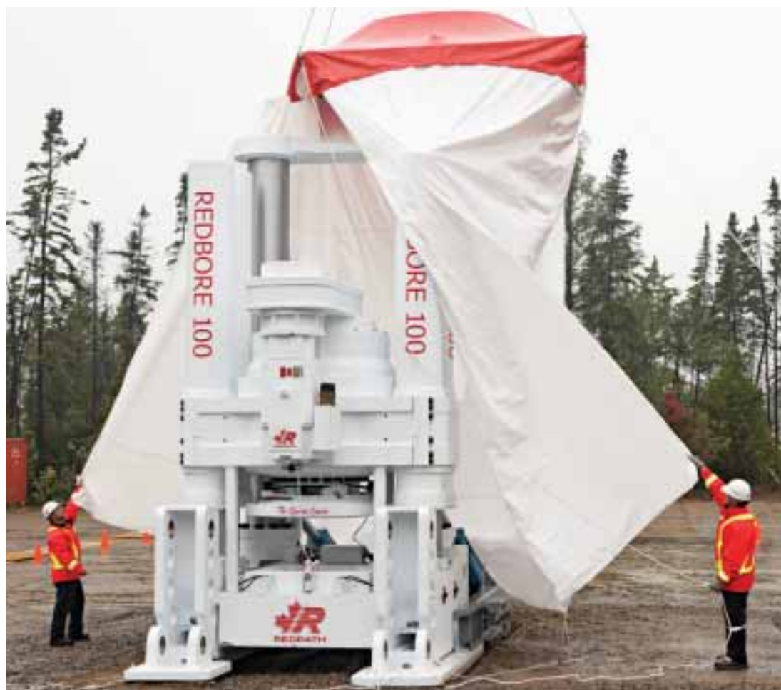
The Redpath Group's Redbore 100 delivers 3.5 million pounds of pull and 750,000 foot pounds of rotational torque.
